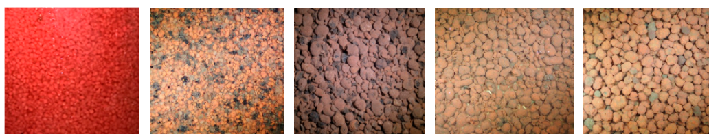
Figure 5. Examples of ANAMMOX granules: AMX only (left) and PN/AMX (4× right) with typical diameters of 1, 1–2, 2–5, 3–5, and 4–6 mm, respectively.
