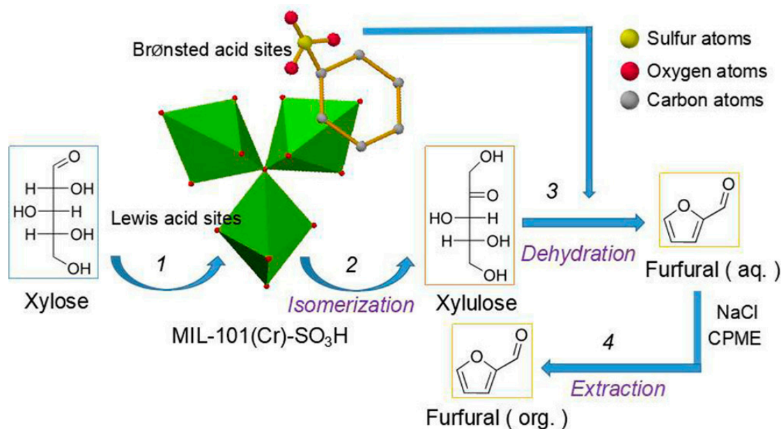
Figure 4. Production of furfural from xylose in the presence of the MIL-101(Cr)-SO 3 H catalyst [64]. Reproduced with permission from Ref. [64].
