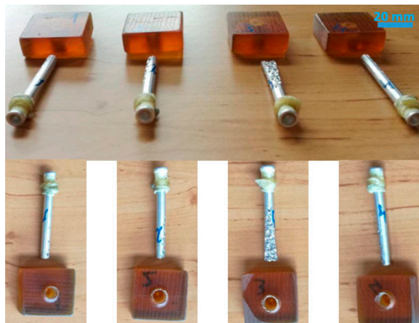
Figure 6. Tested specimens displaying full rivet pullout failure.
