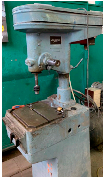
Figure 3. G13 drilling machine used for Friction Riveting.
