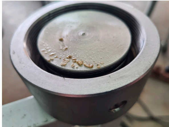
Figure 5. Extract discharge at 8 MPa, no US.
