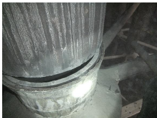
Figure 11. The dipleg fracture in the commercial FCC unit.
