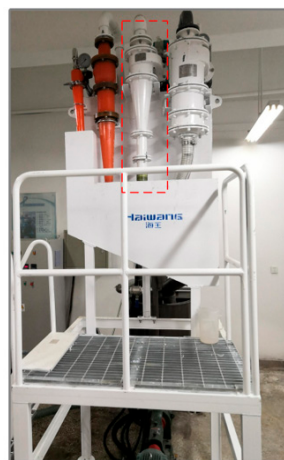
Figure 7. Schematic diagram and implementation of laboratory test rig on the \Phi 150 mm hydrocyclone. 1—Electric cabinet; 2—Mixing tank; 3—Butterfly valves; 4—Centrifugal pump; 5—Magnetic flowmeter; 6—Pressure transmitter; 7—Hydrocyclone; 8—Product sumps.
