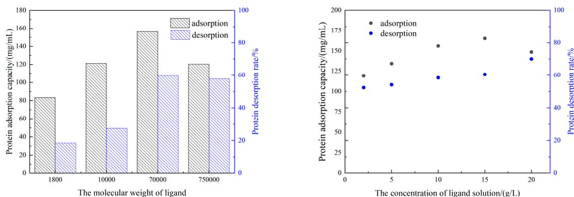
(a) Effect of PEI molecular weight on adsorption/desorption performance
