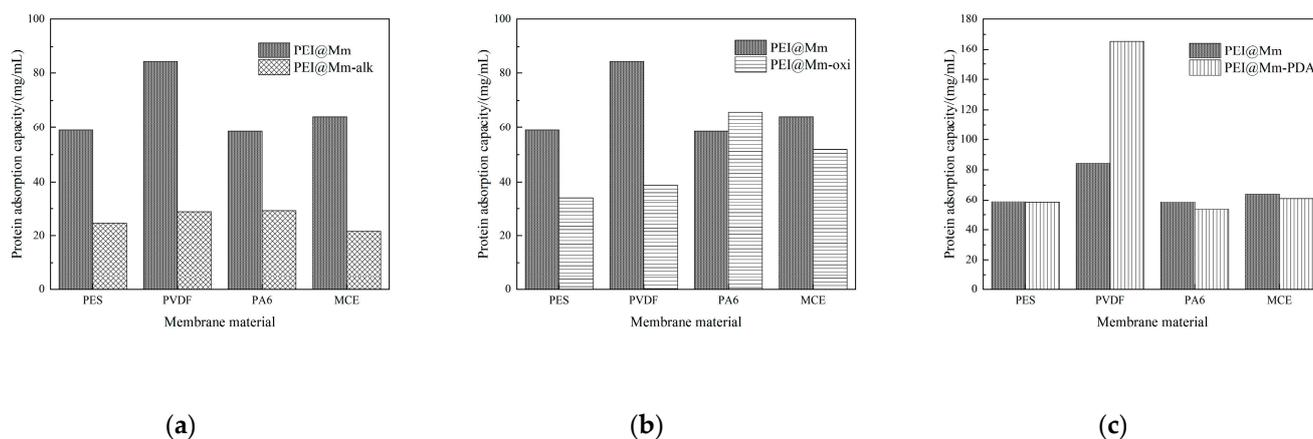
**Figure 5.** Effect of (a) alkali treatment, (b) oxidation treatment and (c) PDA deposition on the protein adsorption performance of the MAs.
