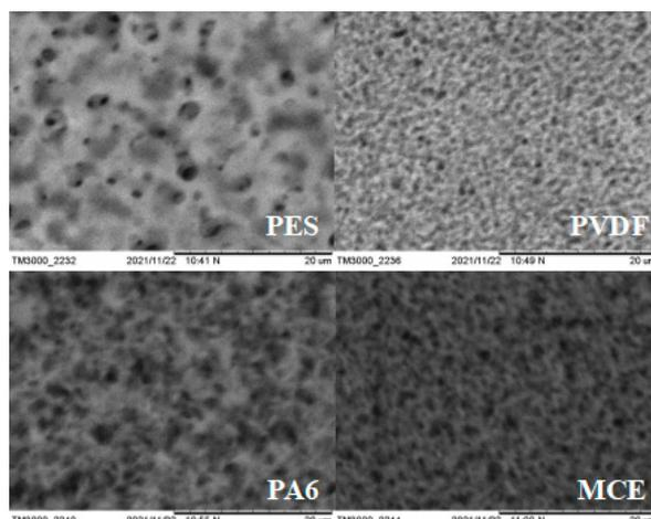
**Figure 6.** SEM images of the surface of pristine PES, PVDF, PA6 and MCE membranes.
