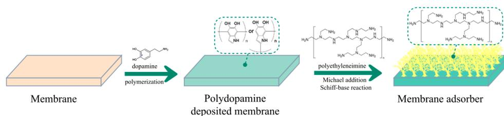
**Figure 1.** Schematic diagram of membrane adsorber prepared by depositing PDA layer on membrane to couple PEI.
