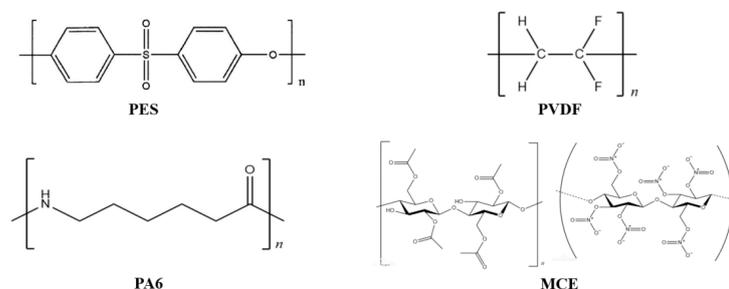
**Figure 2.** The molecular structures of PES, PVDF, PA6 and MCE.
