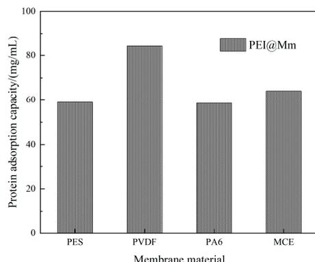
**Figure 4.** Effect of membrane material (different functional groups) on the protein adsorption performance of the MAs.
