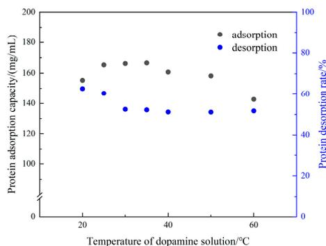
**(b)** Effect of temperature on adsorption/desorption performance
