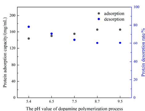
**(a)** Effect of the pH value on adsorption/desorption performance
