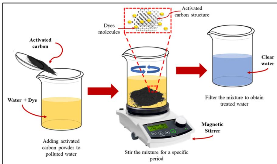
**Figure 16.** Adsorption mechanism of activated carbon for dyes particles.
