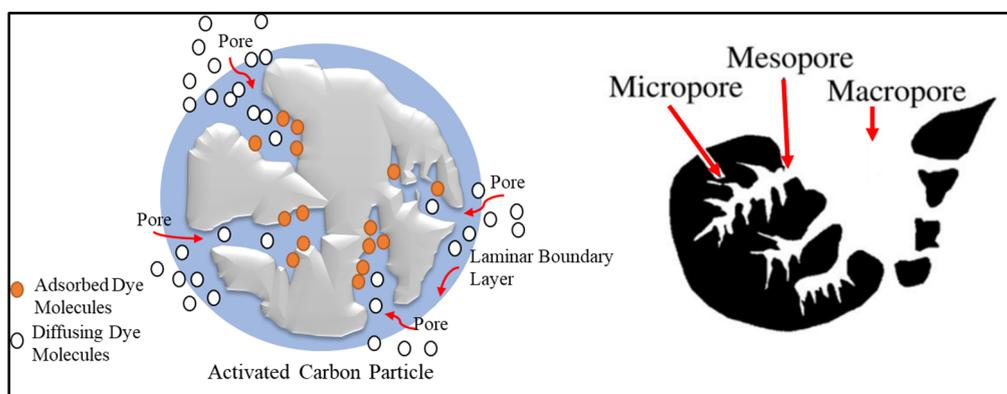
**Figure 14.** Pore structure and distribution on activated carbon.
