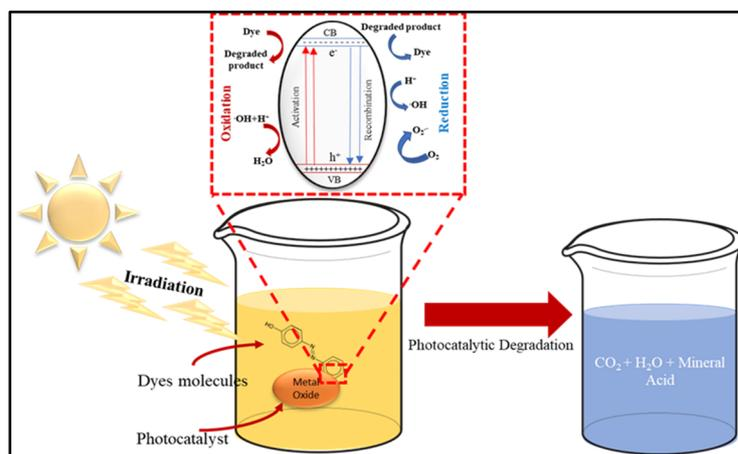
**Figure 13.** Schematic of Photocatalytic Degradation of toxic dye.
