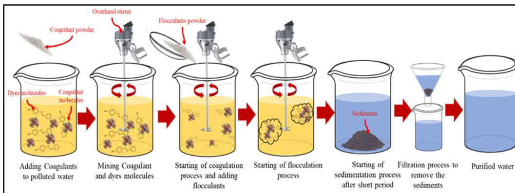
**Figure 11.** Schematic of Coagulation–Flocculation for textile dye wastewater treatment.
