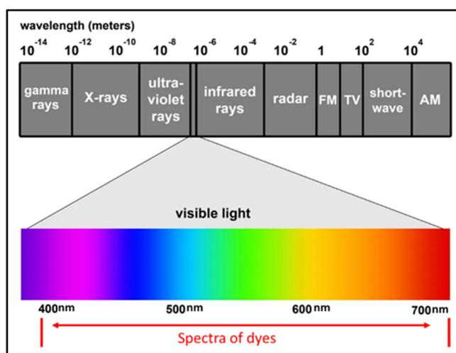
Figure 1. The visible spectrum of colored dyes.
