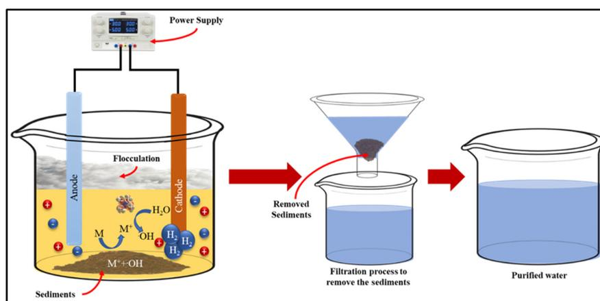
**Figure 12.** Schematic of electrocoagulation for textile dye wastewater.
