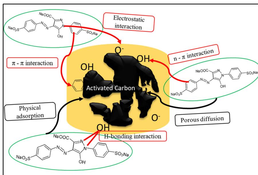
**Figure 15.** Possible mechanisms for adsorbing dyes onto activated carbon.
