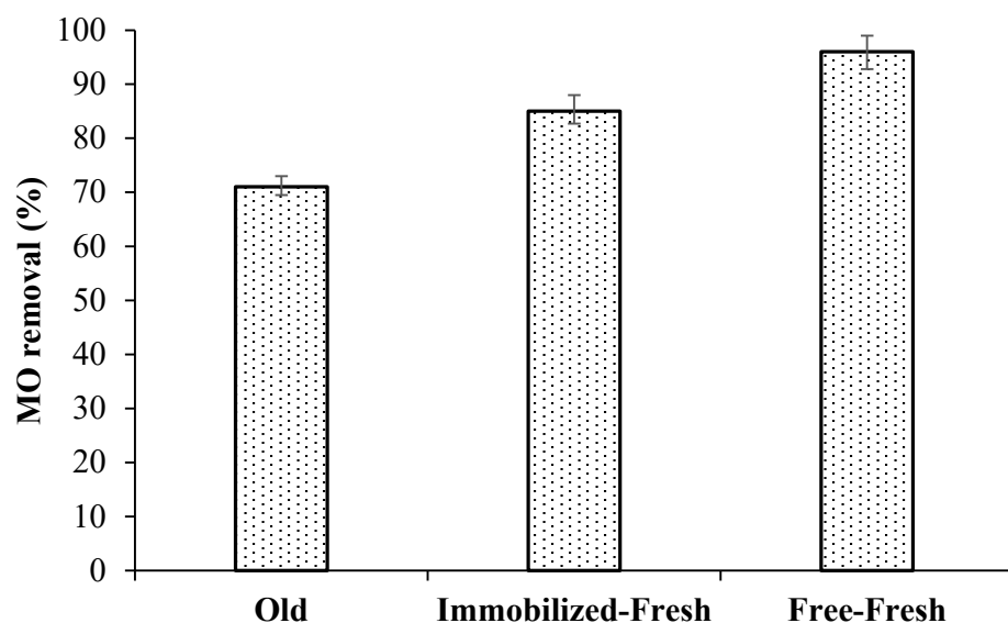
Figure 3. Old, immobilized fresh, and free fresh Bracteacoccus sp. algae for MO dye removal from aqueous solutions. The error bars represent the standard deviation of a triplicate analysis. ( C_o of MO = 10 mg L -1 , adsorbent dose = 0.10 g mL -1 , contact time = 75 min, temperature = 20 °C).
