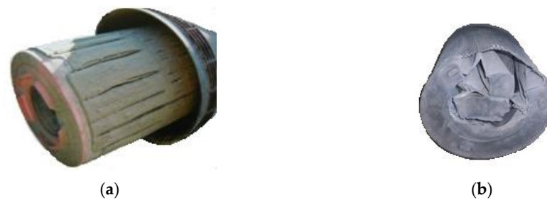
Figure 3. Effects of using air filter after exceeding permissible resistance: (a) excessively contaminated filter element. (b) insert destruction.
