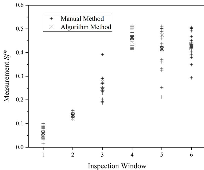
**Figure 5.** Retention values of the six inspection windows of the rotor. Results processed with the automated method are indicated with crosses, plus signs represent manually determined retention values.
