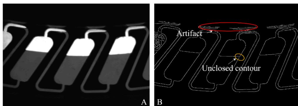
**Figure 2.** (A) Unprocessed still image—extracted from video files of the high-speed camera. (B) Binary image after editing with Canny edge algorithm. Highlighted: Artifact due to reflections (red) and unclosed contour (yellow).
