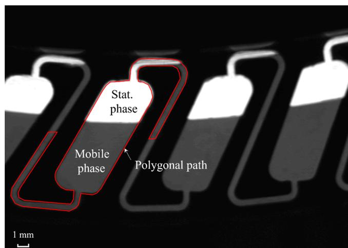
**Figure 1.** Polygonal path (red) highlighting a single chamber-duct combination.
