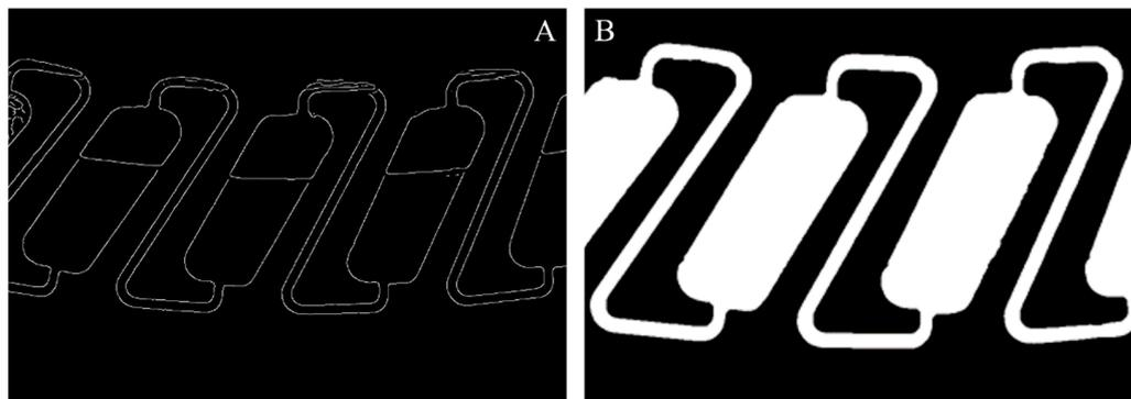
**Figure 3.** (A) Binary image after filtering with the help of a circular mask and edge closure, according to Kovsi. (B) Enclosed areas are filled.
