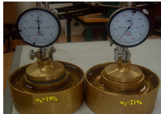
Figure 1. Expansion test of compacted clay after absorbing water.
