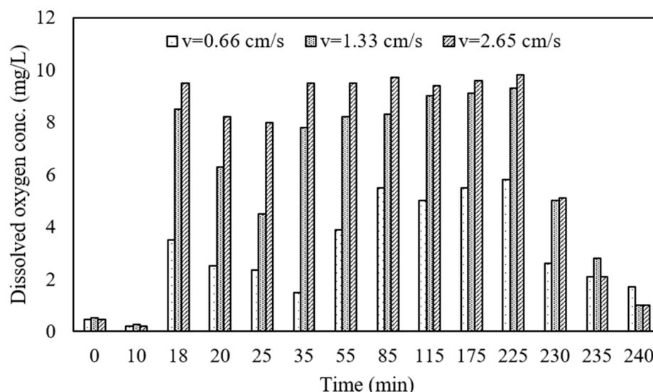
Figure 4. Dissolved oxygen concentration in the reactor at different aeration levels.
