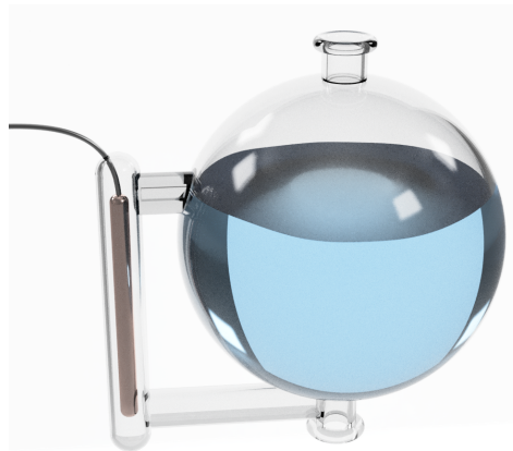
Figure 5. Distillation column boiler.
