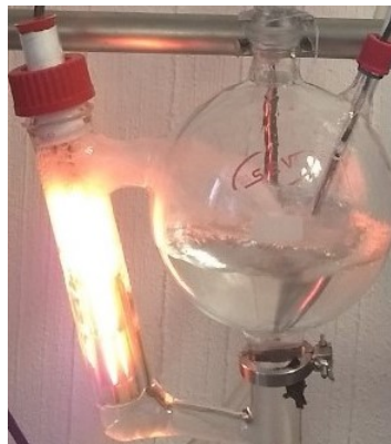
Figure 2. Distillation column heating actuator.
