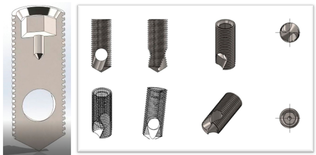
Figure 1. BKS of 4 mm width and 10 mm length, according to the authors project [6].
