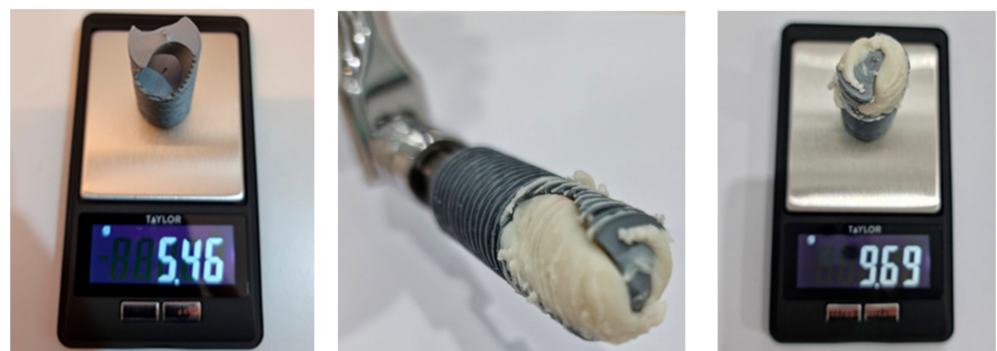
Figure 4. BKS device 3D printed and Taylor Precision Compact Digital scale before and after compacting Aluminum Phyllosilicates (clay).
