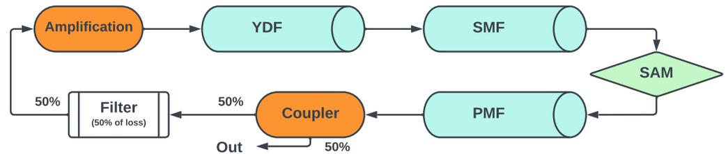
**Figure 3.** The algorithm used for the simulations of the experimental setup. YDF—double-clad Yb-doped fiber, SMF—single-mode fiber, PMF—polarization-maintaining fiber, SAM—self-amplitude modulator.
