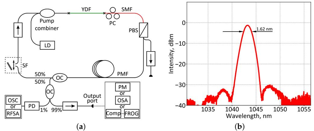
**Figure 1.** Scheme of the experimental setup (a): LD—laser diode, YDF—double-clad Yb-doped fiber, PC—polarization controller, SMF—single-mode fiber, PBS—polarizing beam splitter, PMF—polarization-maintaining fiber, OC—optical coupler, SF—spectral filter, PD—photodiode, OSC—oscilloscope, RFSA—radio frequency spectrum analyzer, PM—power meter, OSA—optical spectrum analyzer, comp—pulse compressor, FROG—pulse duration measurement system; transmission spectrum of the spectral filter (b).
