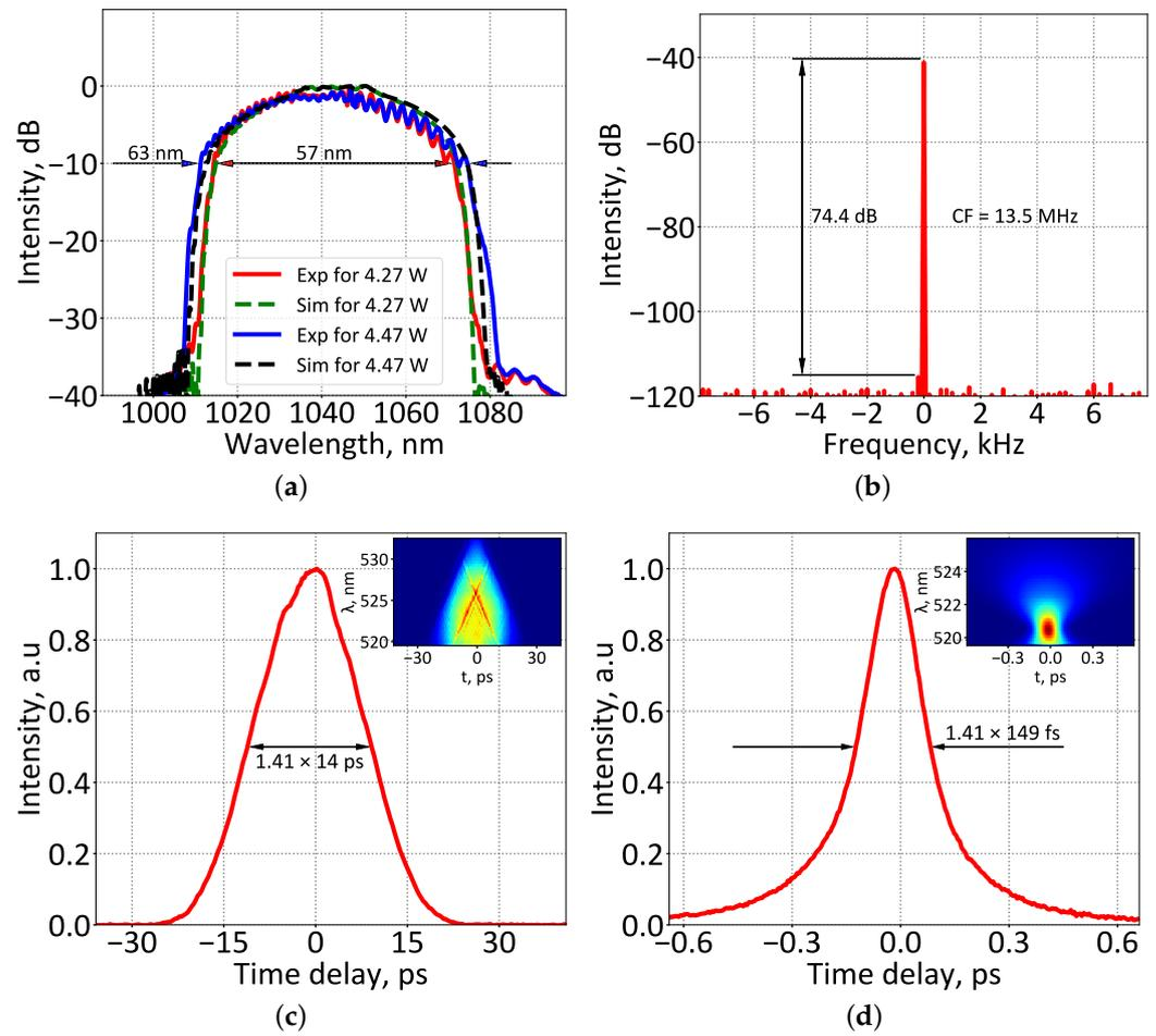
**Figure 2.** Parameters of the pulses: normalized optical spectra for the 4.3 W of the pump power (solid red line) and 4.5 W (solid blue line), the dashed lines represent the results of numerical simulations (a); RF spectrum (b), CF—central frequency; autocorrelation function with corresponding FROG trace (inset) for the chirped pulse (c) and compressed one (d).
