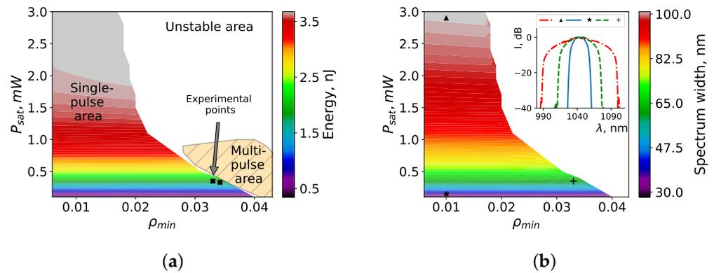
**Figure 5.** Parameters of the pulses of stable area: energy of single-pulse and multi-pulse areas (a) and spectrum width at the level of  $-10$  dB (b). The crosses indicate the regimes corresponding to the experiment. Inset: spectral shapes in points marked by triangle, star, and cross.
