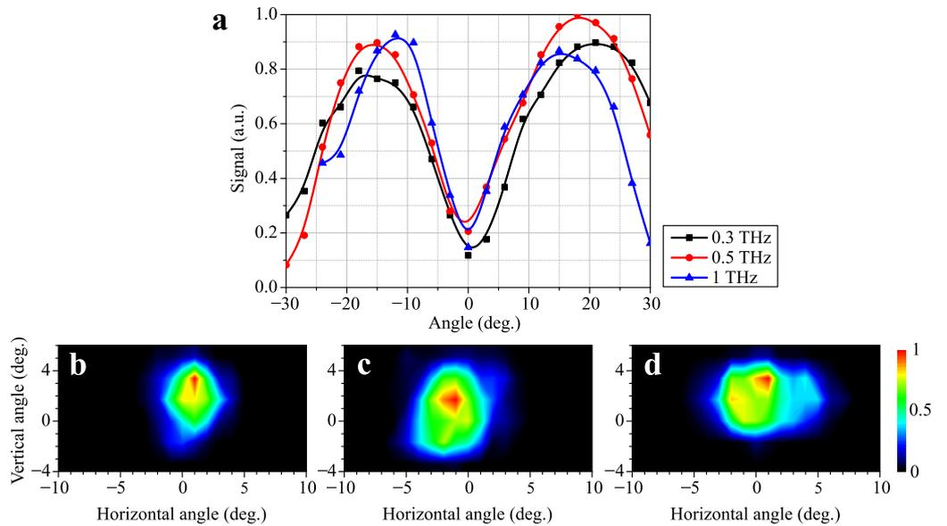
**Figure 3.** Normalized angular distribution of terahertz radiation without the pipe (a) and with the use of the polypropylene pipe for frequencies: 0.3 THz (b), 0.5 THz (c) and 1 THz (d). The focal length is 20 cm, laser pulse energy is 10 mJ.
