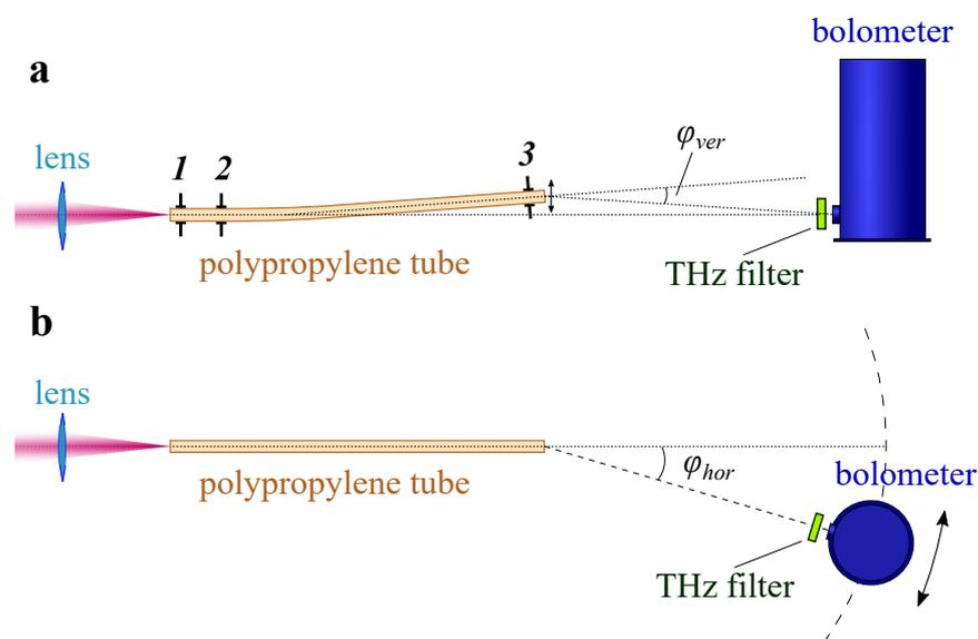
**Figure 1.** Scheme of the experiment: (a) side view; (b) view from above. 1–3—mounts fixing the pipe.
