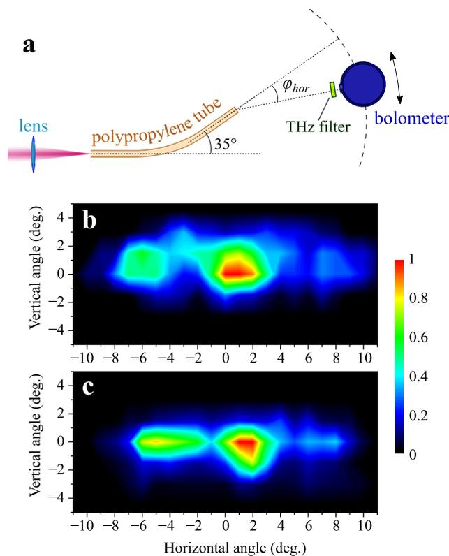
**Figure 4.** Scheme of the experiment with the bent pipe (a). Angular distribution of the radiation with frequencies of 0.5 THz (b) and 1 THz (c) passed through the bent pipe.
