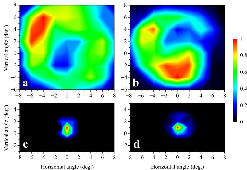
**Figure 2.** Normalized angular distributions of the radiation with frequencies of 0.5 THz (a,c) and 1 THz (b,d), without (a,b) and with (c,d) the polypropylene pipe. Focal length is 1 m, laser pulse energy is 3 mJ.
