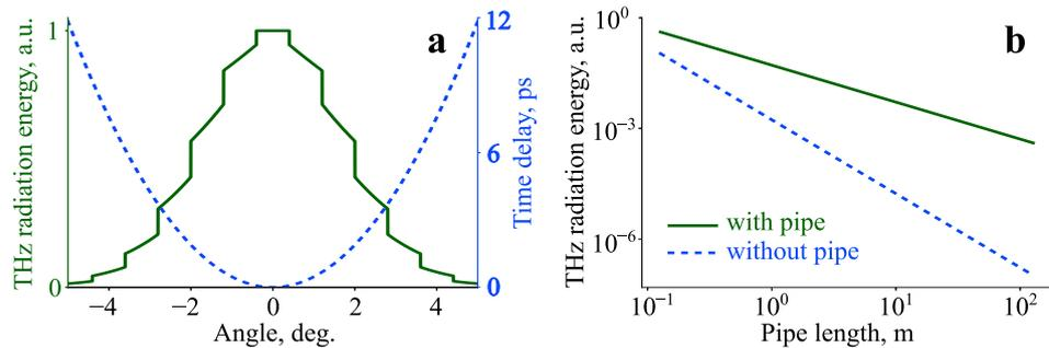
**Figure 5.** Terahertz radiation angular distribution at the pipe output (green solid line) and delay of the terahertz pulse depending on the propagation angle (blue dashed line) (a). Energy of terahertz radiation contained in the aperture corresponding to the pipe diameter depending on the distance for free propagation and propagation in the pipe (b).
