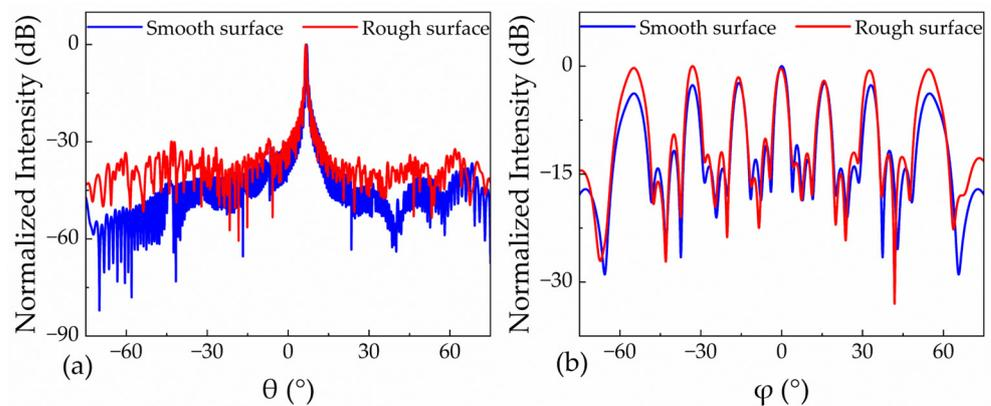
Figure 3. Far-field distribution of Si antennas with smooth and rough surface morphologies is shown in (a) the  $\theta$  direction and (b) the  $\varphi$  direction.
