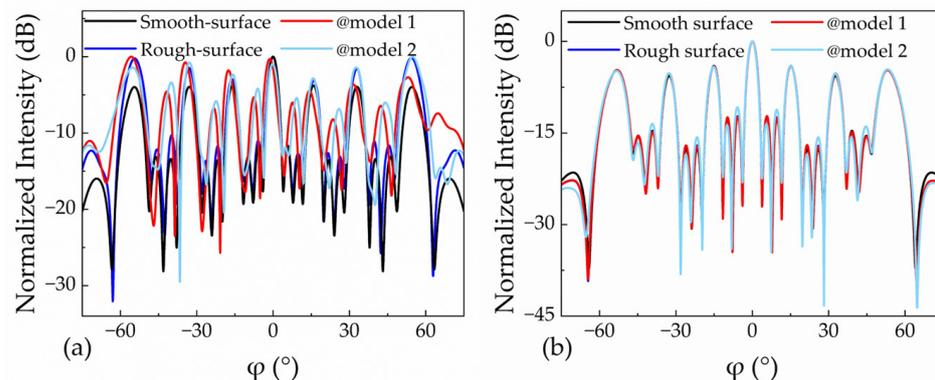
**Figure 5.** Far-field energy distribution in  $\varphi$  direction after introducing errors in the width and the thickness into antennas: (a) Si antenna; (b)  $\text{Si}_3\text{N}_4$  antenna.
