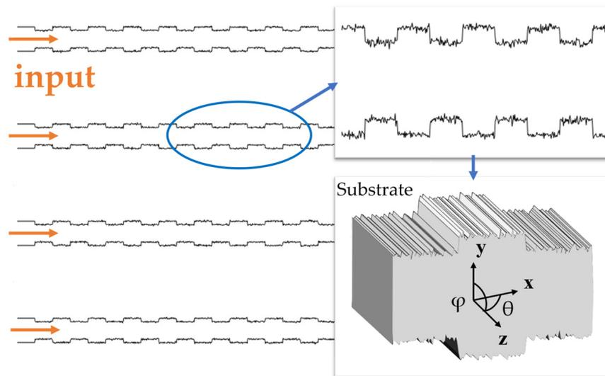
Figure 2. Sketch map of the rough burr surface on both sides of the antenna (array).
