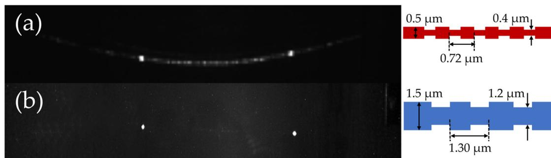
**Figure 1.** Far-field experimental results and detailed parameters of (a) Si and (b)  $\text{Si}_3\text{N}_4$  antennas.
