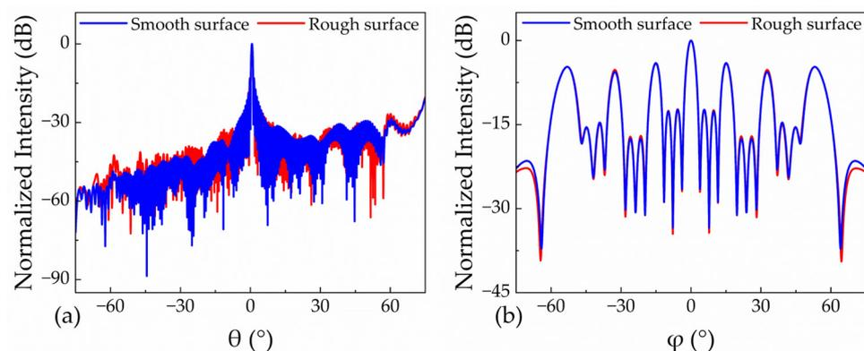
**Figure 4.** Far-field distribution of Si<sub>3</sub>N<sub>4</sub> antennas with smooth and rough surface morphologies (a) in the  $\theta$  direction; (b) in the  $\varphi$  direction.
