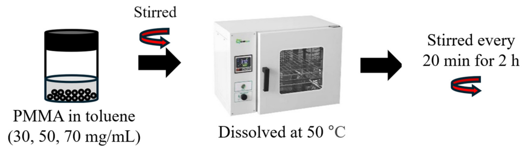
Figure 4. Fabrication of coating material.
