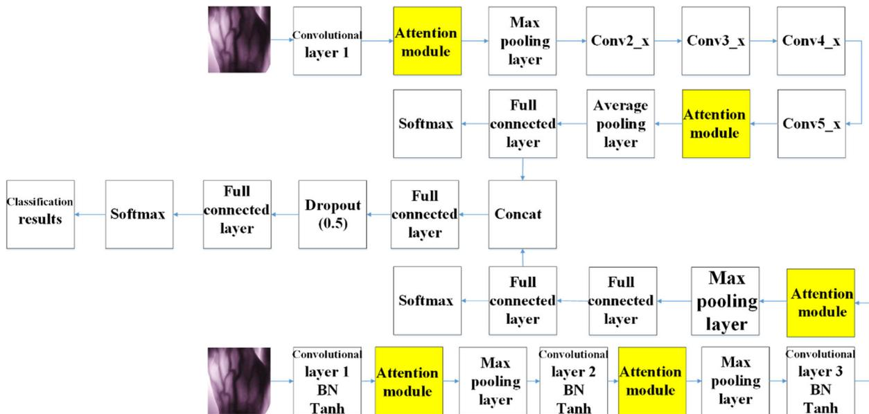
Figure 4. The framework of the dual-stream enhanced network with an attention mechanism (DSEANET).
