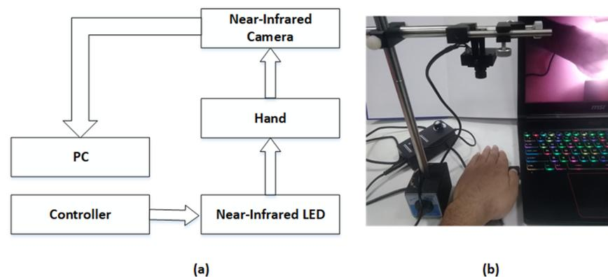
**Figure 1.** The schematic diagram and three-dimensional layout of near-infrared dorsal hand vein capturing system [15]. (a) the component diagram; and (b) the physical image.
