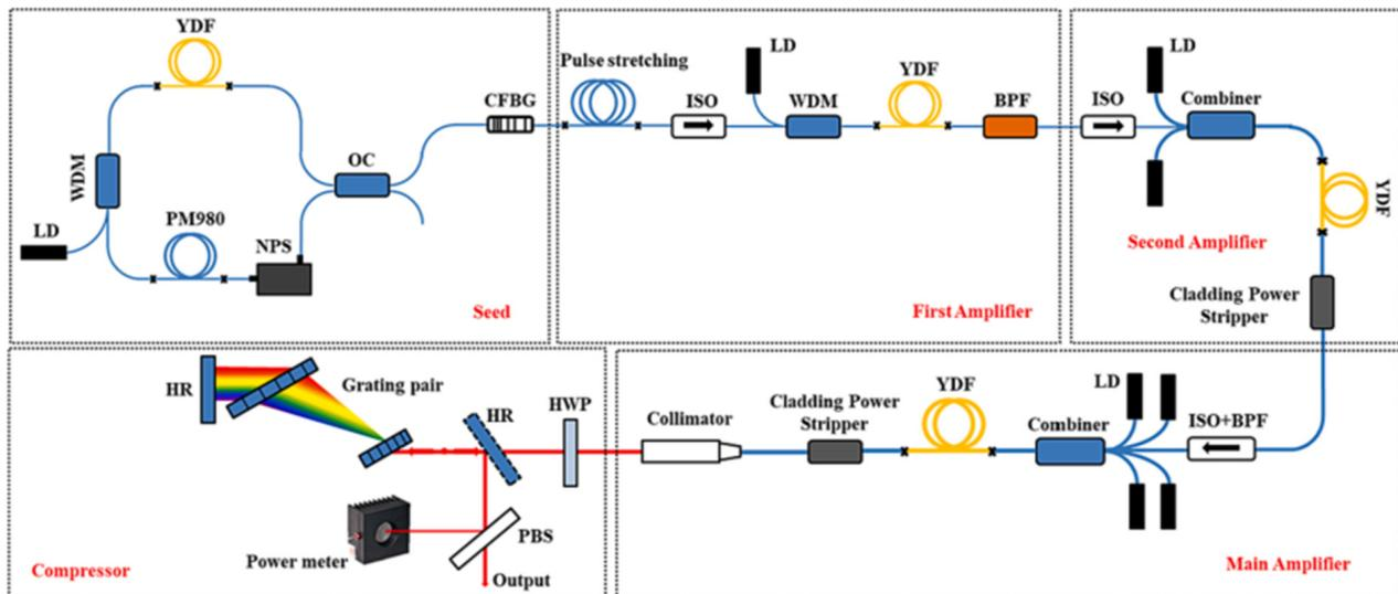
**Figure 3.** Schematic of the proposed CPA system. OC, coupler; NPS, nonlinear phase shifter [27].
