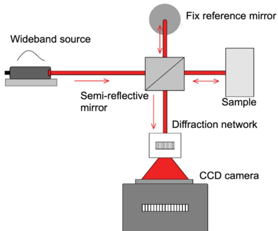
**Figure 2.** Schematic of OCT [19].
