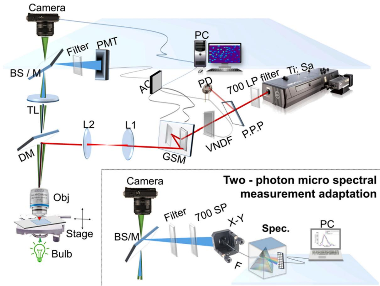
**Figure 4.** Schematic 3D drawing of the home-built TPEF microscope with specific adaptations for in situ emission spectra measurement [22].
