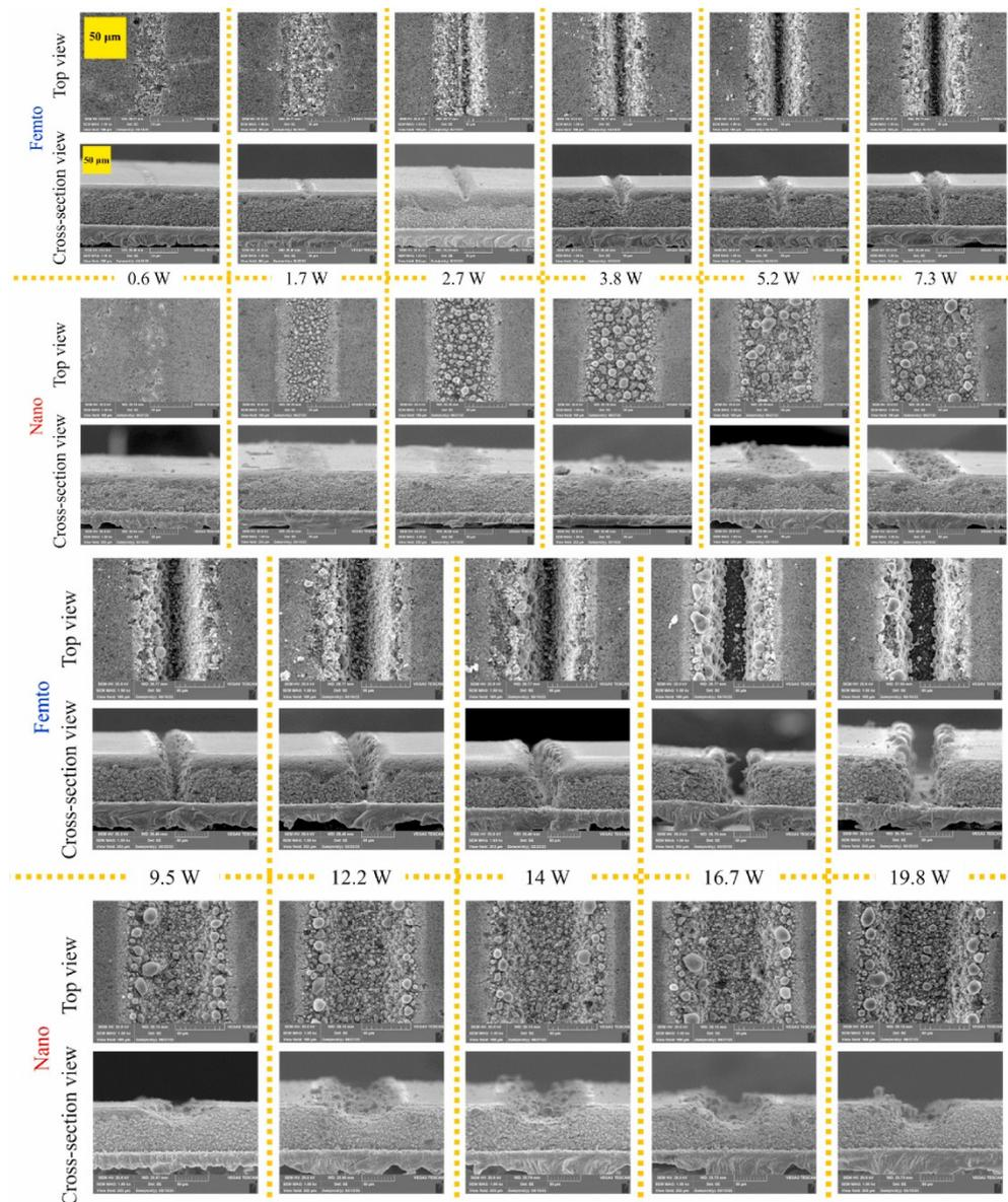
**Figure 1.** Material processing by an ultrafast laser and comparison with a nanosecond laser [1].
