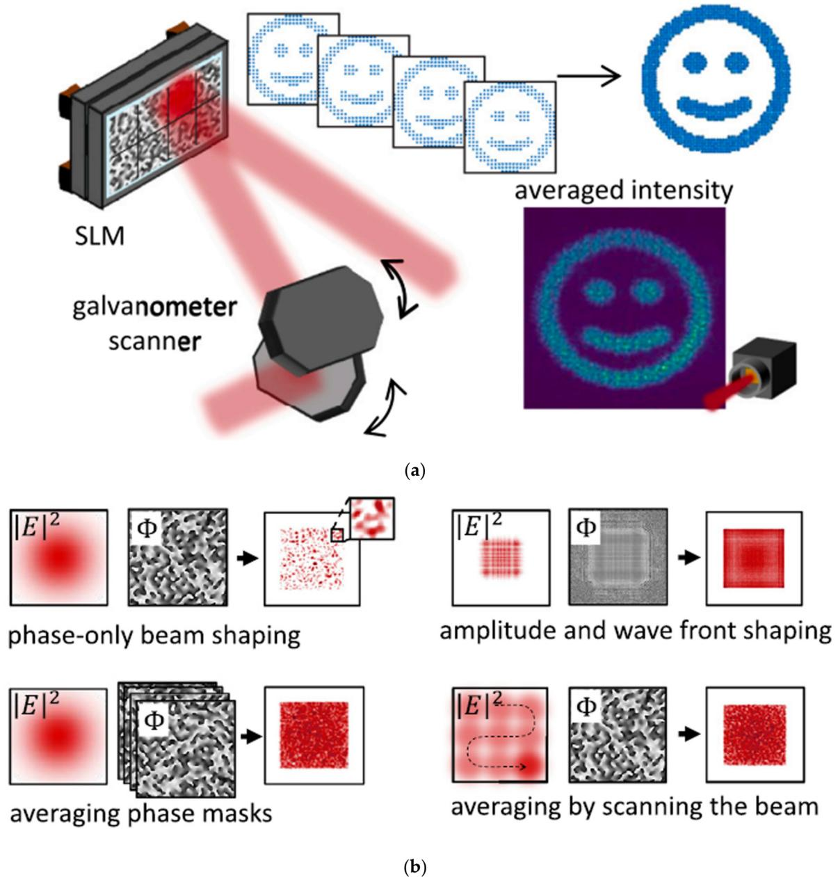
Figure 5. (a) SLM for spatial beam shaping. (b) Methods for phase-only beam shaping [26].
