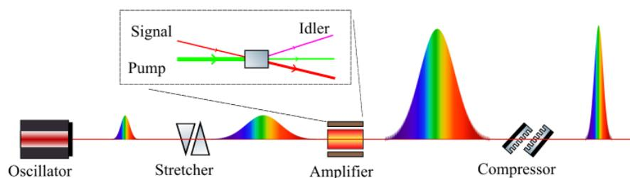
**Figure 2.** Schematic process of Optical Parametric Chirped Pulse Amplification. The low-power, short pulse is stretched, parametrically amplified, and then compressed to achieve a high-power short pulse. An idler beam is created as a result of the phase-matching in the amplification.
