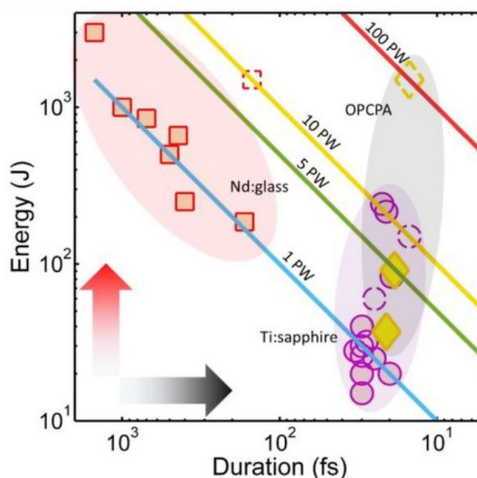
**Figure 1.** Potential and achieved power of laser pulses based on amplification medium (reprinted with permission) [44]: red symbols represent Nd:Glass systems; purple Ti:Sapph; and yellow OPCPA. Solid and dashed outlines indicate complete facilities and lasers in construction respectively.
