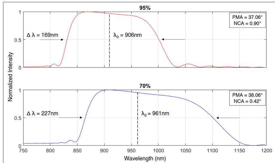
**Figure 3.** Simulated bandwidth  $\Delta\lambda$ , central wavelength  $\lambda_0$ , phase matching angle (PMA), and non-collinear angle (NCA) based on DKDP deuteration levels of 95% and 70%, using the Sellmeier equations for DKDP [41].
