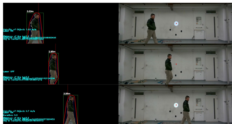
Figure 7. The 3-stage process of a single intrusion object, including the approaching Safety-Distance area, passing through the light beam and leaving the safety area.
