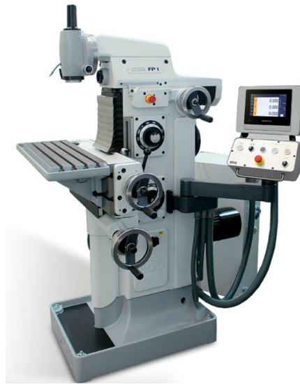
Figure 9. Refurbished DMG MORI AG milling machine. This type of machine is already fitted with glass scale linear encoders in the three main axes, with each having an accuracy of 5\ \mu\text{m} . Fortunately, in each one of the three main directions, there is a sufficiently large amount of space to add a movable mirror and a fixed InGaAs/InAlAs-based, monolithically integrated interferometer chip.
