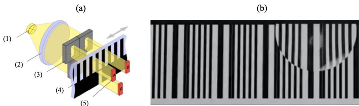
Figure 8. Schematic view (a) and short section (b) of a glass scale linear encoder, as is used today in state-of-the-art CNC machines. Such encoders have a positioning accuracy of 5 \mu\text{m} [47]. (1) LED light source, (2) condenser lens, (3) slit mask, (4) glass ruler, and (5) photodetectors.
