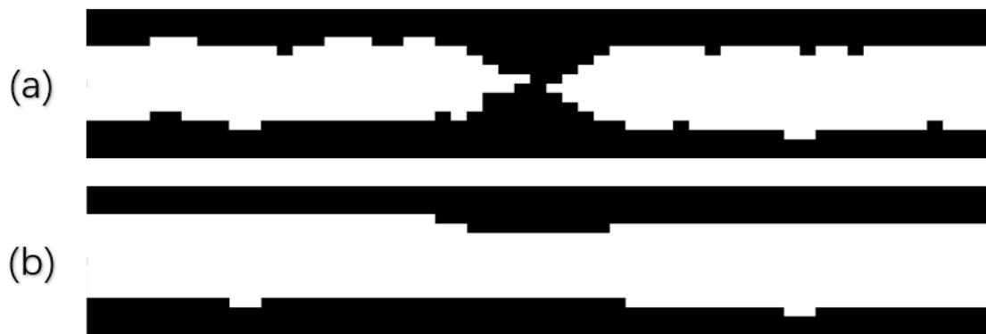
Figure 1. Mask images of the region of interest extraction. (a) after threshold segmentation; (b) after closing operation.
