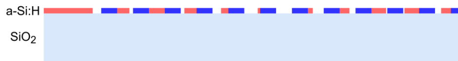
Figure 15. Grating coupler made from the superposition of two diffraction gratings with periods of 1500 nm (represented in red) and 1300 nm (represented in blue). The result is a grating with a chaotic (random) distribution.
