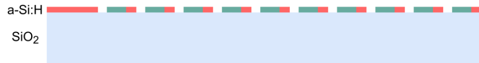
Figure 14. Grating coupler made from the superposition of two diffraction gratings with a period of 1500 nm; the result is a grating with the same period and a fill factor of 76.(6)%. Grating segments with and without offset are represented by the colors green and red, respectively.
