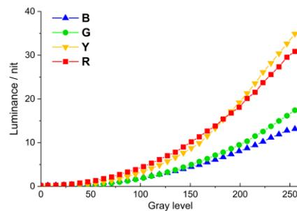
Figure 1. Gamma curves of the four primaries.
