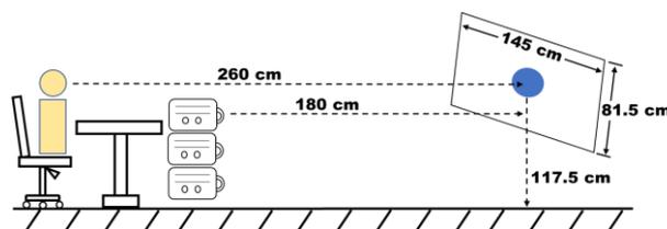
Figure 9. Experimental setup.
