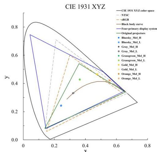
Figure 3. Experimental stimuli and colour gamut of the display system and the original projectors.
