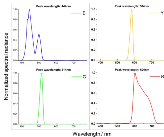
Figure 2. Spectra of the four primaries.
