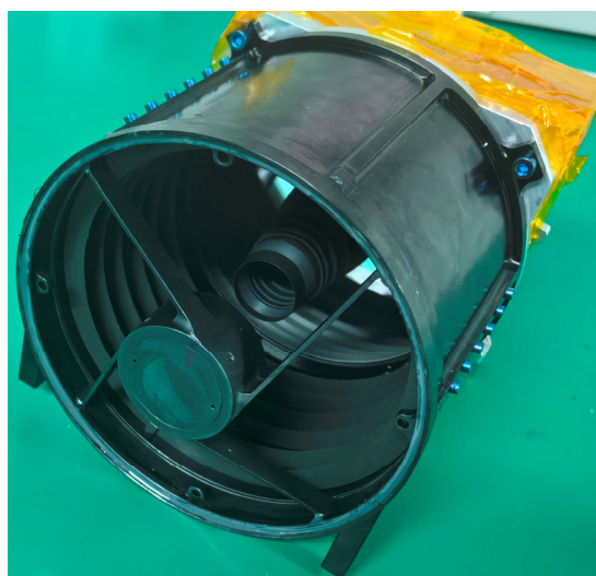
Figure 6. Image of the camera’s optical objective lens.
