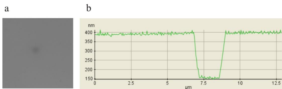
Figure 6. (a) Image of our sample detected by the CCD camera in white light; (b) scan of the square profile taken with the Atomic Force Microscope. The sample was etched in a polymer with refractive index n = 1.49 .
