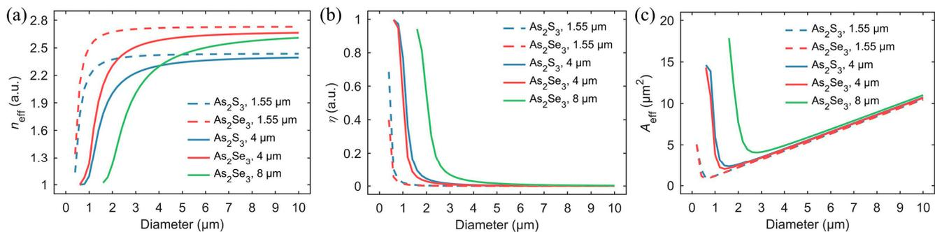
**Figure 2.** Numerical solutions of diameter-dependent (a) effective refractive index ( $n_{\text{eff}}$ ), (b) fractional evanescent fields ( $\eta$ ), and (c) effective mode area ( $A_{\text{eff}}$ ) of  $\text{As}_2\text{S}_3$  and  $\text{As}_2\text{Se}_3$  MFs at wavelengths of 1.55  $\mu\text{m}$ , 4  $\mu\text{m}$ , and 8  $\mu\text{m}$ , respectively.
