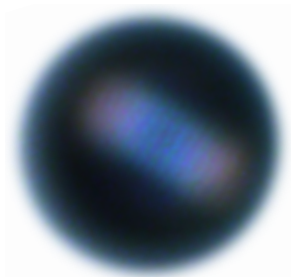
Figure S1. Optical microscopic image of a Blu-ray disc observed under a bright-field reflection microscope through a patchy BaTiO 3 microsphere which has a diameter of 35 \mu\text{m} and is partially coated with 100 nm-thick aluminum thin films.
