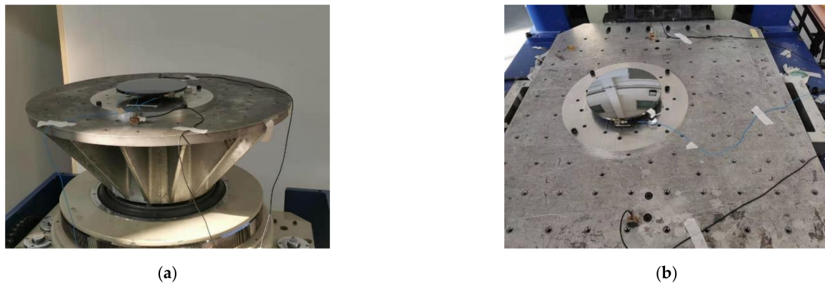
Figure 14. The test of mechanical vibration: (a) Z-direction vibration (axial) (b) Y-direction vibration (lateral).
