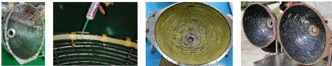
Figure 10. The installation of the photovoltaic cell.
