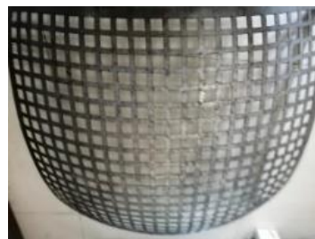
Figure 4. The deformed holes after stamping.
