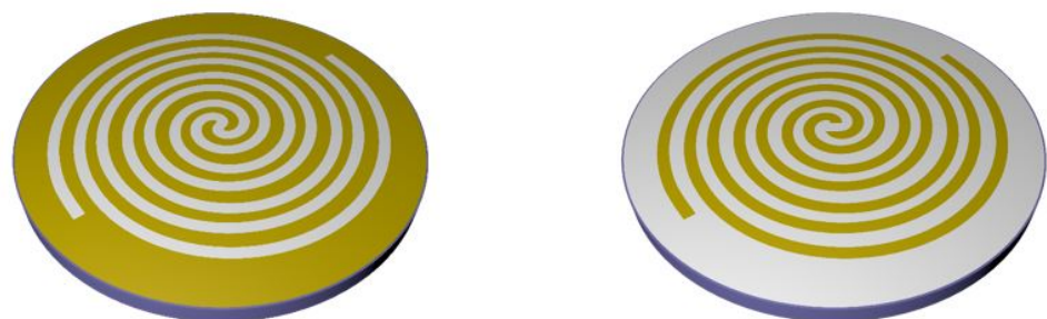
Figure 6. Slot-spiral structure (left) and spiral structure (right) both integrated with high-electron-mobility transistor (HEMT) in the center.
