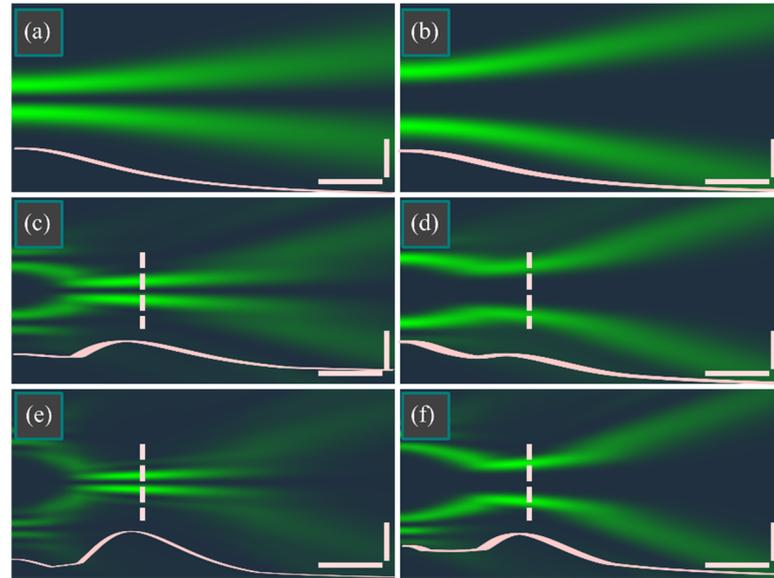
**Figure 3.** Longitudinal intensity distributions of the beam from Equation (1) with the topological charge of 1 (**a,c,e**) and 4 (**b,d,f**) when the radial (lower) index  $n$  of the associated Laguerre polynomial is as 0 (**a,b**), 3 (**c,d**), 6 (**e,f**). Below each distribution, a longitudinal intensity cross-section is shown. Horizontal and vertical scale marks denote, respectively,  $z_0/2$  and 1 mm. Transverse dashed line denotes the autofocus plane  $z = z_0$ .
