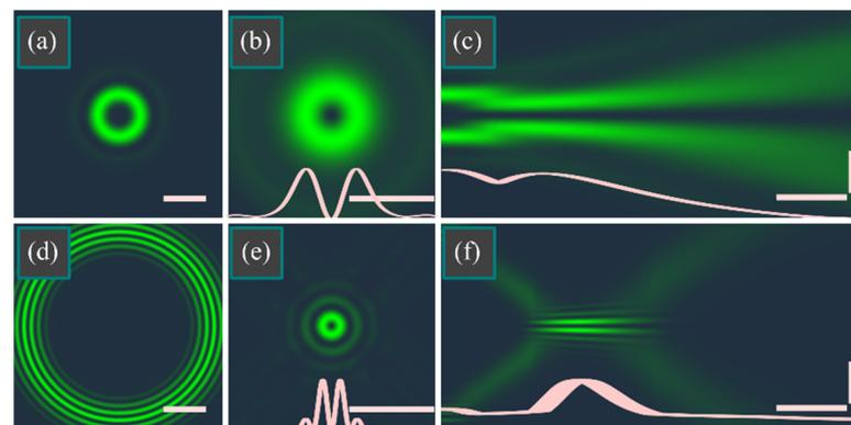
**Figure 4.** Transverse initial (**a,d**) and focal (**b,e**) intensity distributions, as well as the longitudinal intensity distributions (**c,e**) of the beam from Equation (1) with the  $(n, m) = (1, 2)$  (**a–c**) and with the  $(n, m) = (20, 21)$  (**d,f**). Curves (**b,c,e,f**) show the intensity cross-sections. Horizontal scale marks in the transverse patterns denote 1 mm. Horizontal and vertical scale marks in longitudinal patterns denote  $z_0/2$  and 1 mm, respectively.
