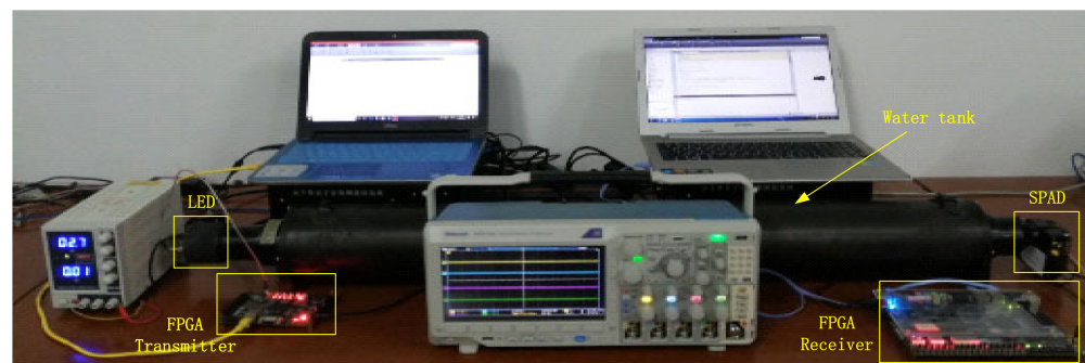
Figure 11. Diagram of the water tank experimental system.
