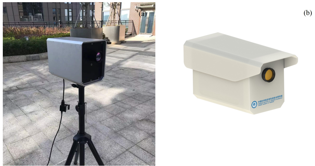
Figure 2. (a) Physical view of broadband infrared spectral imaging system; (b) Rendering picture of broadband infrared spectral imaging system.
