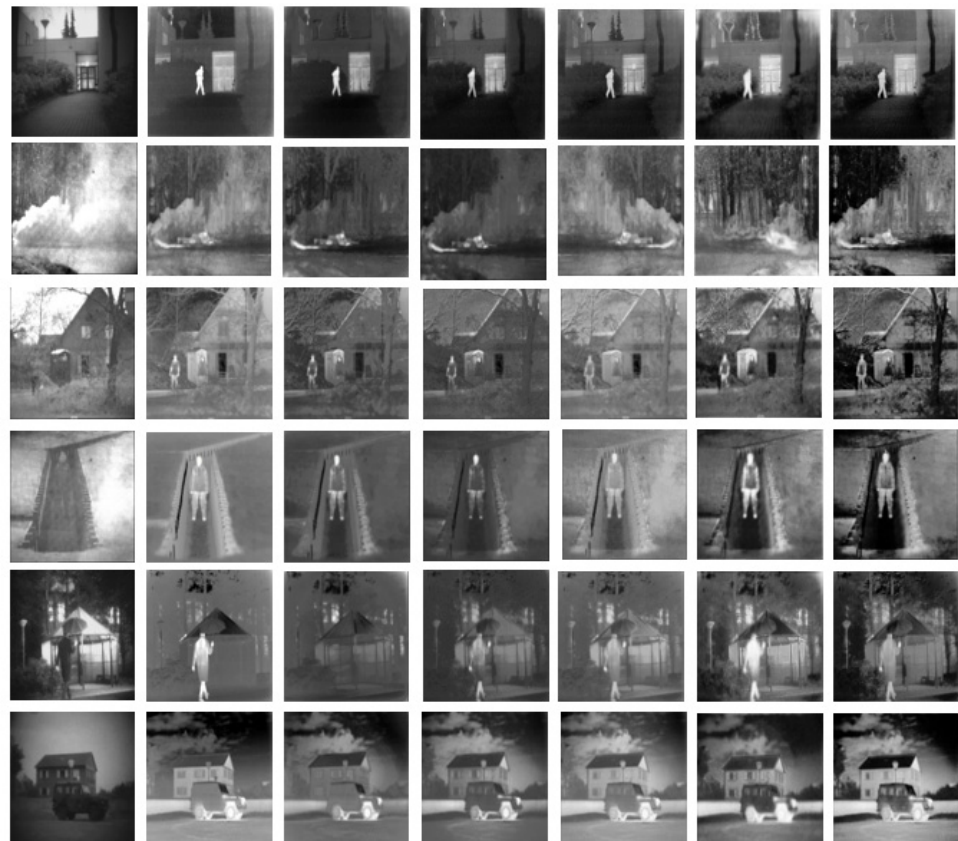
Figure 5. Qualitative results for the TNO dataset. From left to right: visible images, infrared images, and fused results with FusionGAN, GANMcC, PMGI, DDCGAN, and DDGANSE (Ours).
