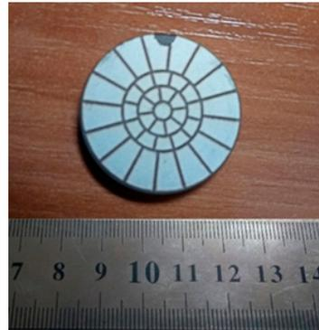
**Figure 2.** The electrode grid placed on the piezodisk surface.
