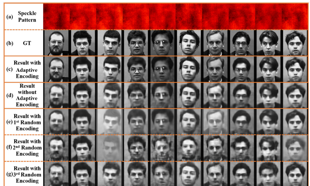
Figure 7. Comparison of AESINet-R reconstruction results with different encoding methods. (a) The Speckle pattern. (b) The Ground Truth (GT) of the hidden target. (c) AESINet-R test set reconstruction results after adaptive encoding by AESINet-E. (d) The AESINet-R reconstruction result when the speckles without adaptive encoding as input. (e–g) The AESINet-R reconstruction result after speckle is modulated by randomly generated gaussian encoding mask.
