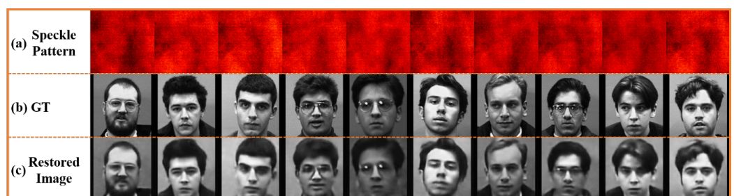
Figure 5. The reconstruction result of the face data set by AESINet. (a) The Speckle pattern. (b) The Ground Truth (GT) of the hidden face. (c) The reconstruction results by using adaptive coding.
