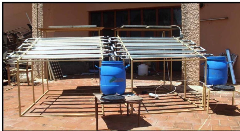
Figure 24. Fixed-bed tubular reactor for purification of rainwater. (Reprinted/adapted with permission from Ref. [114]).
