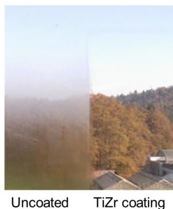
Figure 18. Antifogging effect of uncoated and TiZr coated glass. (Reprinted/adapted with permission from Ref. [23]).
