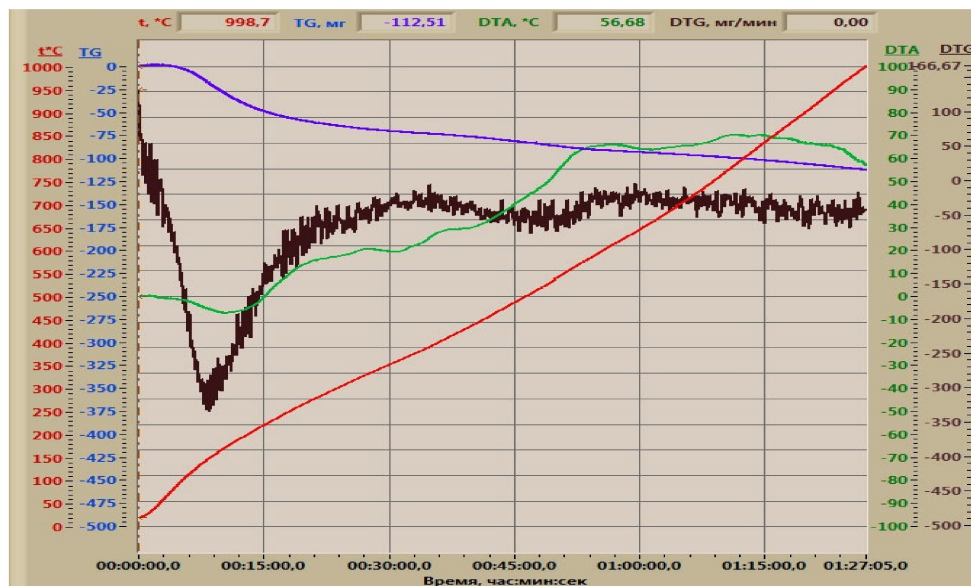
Figure 3. Derivatogram (DTA) of cottrel dust.
