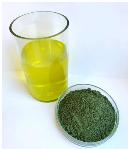
Figure 1. Liquid and solid phases of catalyst slurry.
