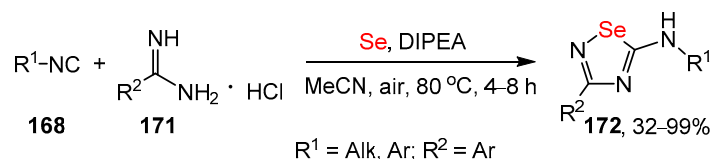
Scheme 67. Synthesis of 1,2,4-selenadiazol-5-amine derivatives 172 by three-component reaction of isocyanides 168 , arylamidinium hydrochlorides 171 and elemental Se.
