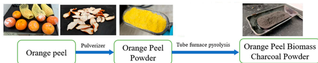
Figure 11. Schematic diagram of the preparation of orange peel biocarbon materials.
