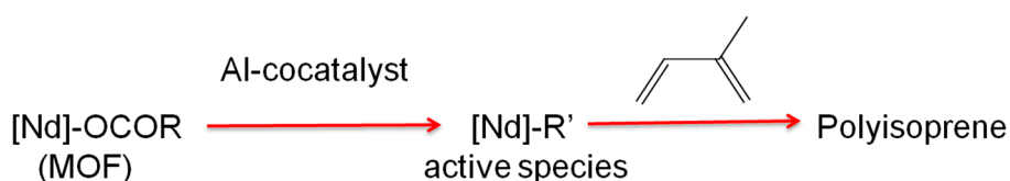
Scheme 1. The activation of the catalyst by the combination of a MOF pre-catalyst and alkyl-aluminum co-catalyst.
