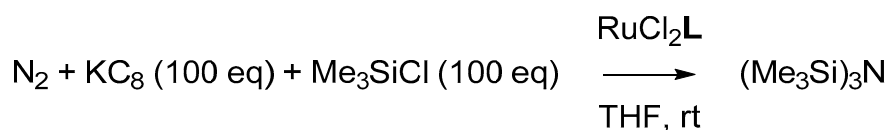
Figure 11. Reduction of dinitrogen with KC 8 , Me 3 SiCl and RuCl 2 L forming (Me 3 Si) 3 N.
