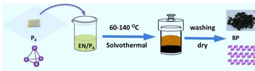
Figure 6. Schematic representation of the synthesis of few-layer BP nanosheets through a solvothermal process at the temperature range of 60–140 °C using white phosphorus as raw material and ethylenediamine (EN) as solvent [41].
