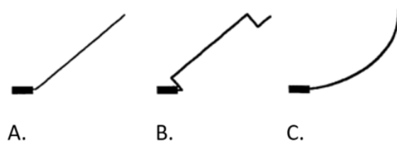
Figure 2. Cantilever design: (A). tip-back (TB) (B). utility arch (UA) (C). deep curve (DC).
