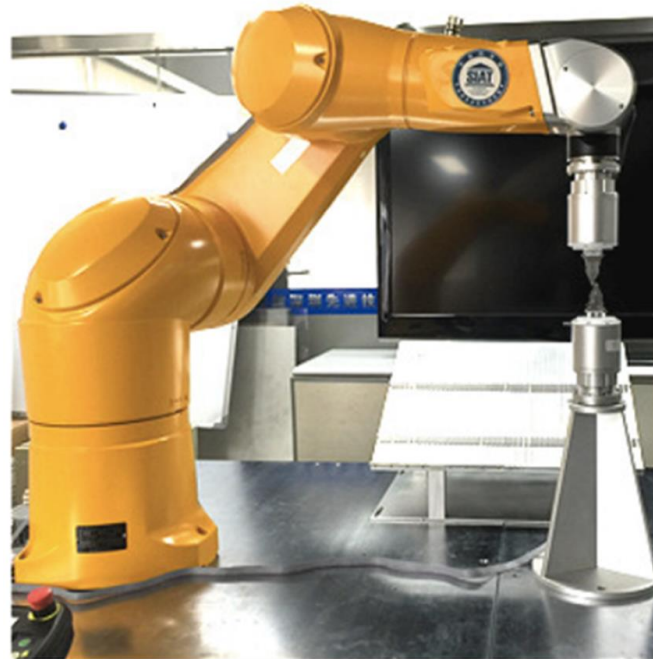
Figure 5. Novel robot system for orthodontic archwire bending [38].
